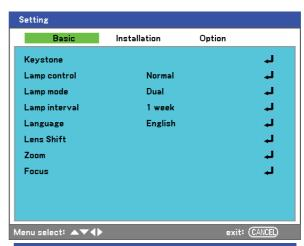
From the Lamp control window, select Normal or Eco using ▲or▼. Select OK and press ←.
